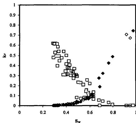
Figure 8. Experimental results from Mahiya (1999) adiabatic experiment. Closed symbols, drainage curves; open symbols, imbibition curves.
