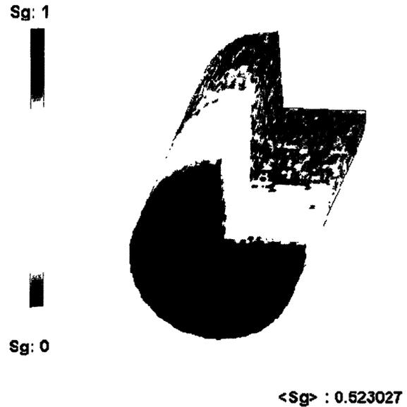
Figure 2. Steam distributions measured by X-ray CT, from Satik (1998).
