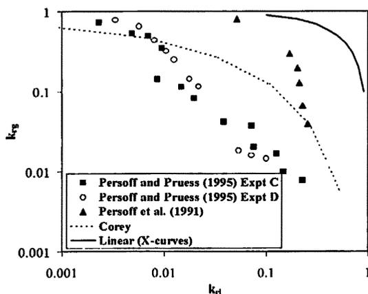
Figure 12. Some measurements of air-water relative permeabilities in rough-walled fractures.
