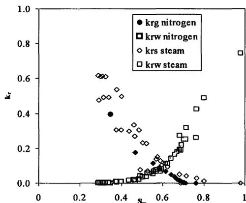
Figure 10. Comparison between steam-water (open symbols) and nitrogen-water imbibition (closed symbols) relative permeabilities on the same rock core.
