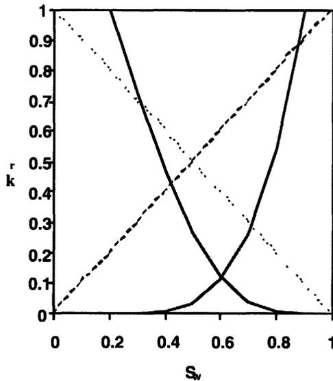
Figure 1. Corey (solid lines) and linear (dashed lines) relative permeability curves.
