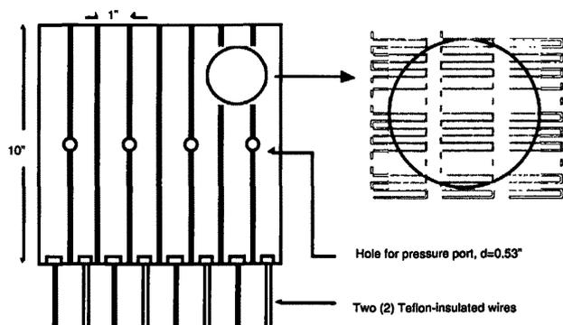
Figure 7. Schematic of flexible heaters.
