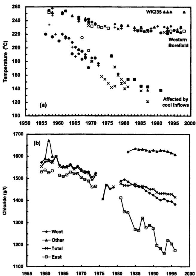
Figure 5a. Trends in average temperature from liquid feedzones in Wairakei production areas; b. Trends in average corrected chloride concentrations from the Wairakei production areas (from Glover, 1998).
