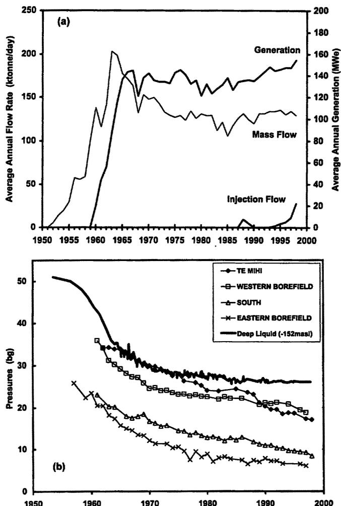
Figure 3. Upper graph shows the production history of the Wairakei power plant, along with the average annual production and injection mass flows. Lower graph shows the trend in pressure of the liquid reservoir at a datum approximately equivalent to 550 m depth (bold line), and the trends in steam-zone vapour pressure in different sectors of the field.
