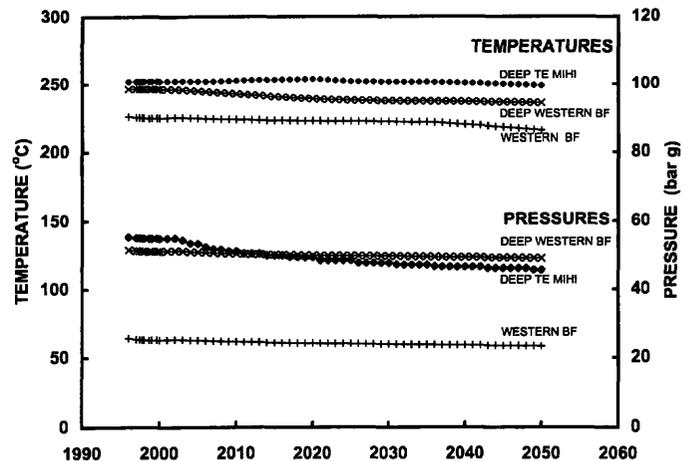
Figure 6. Model prediction of the future production trends at Wairakei assuming 60% of the production mass in injected, and make-up production wells are located in Te Mihi. The model is by O'Sullivan *et al.* (1998).
