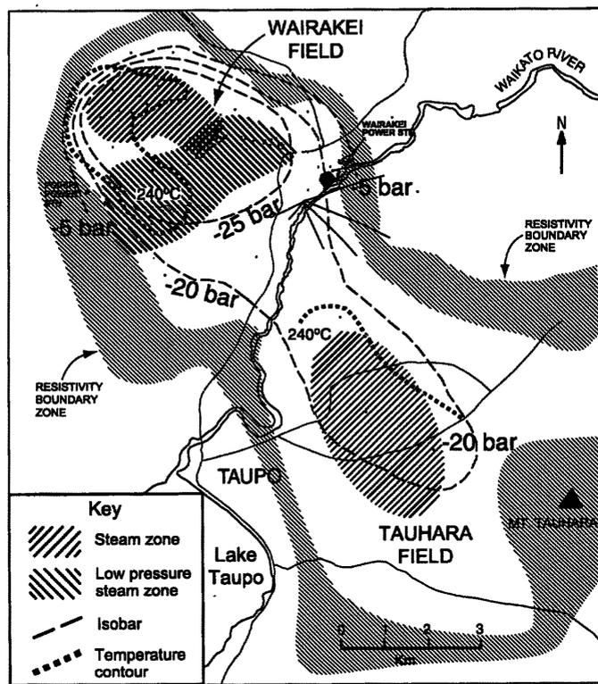
**Figure 4.** Compilation from the mid 1990s of the extent of pressure decline in the liquid reservoir, the known areas of highest temperature at about 800 m depth (> 240°C at -400 m asl), and the locations of the steam zones which have formed as a result of the pressure decline.
