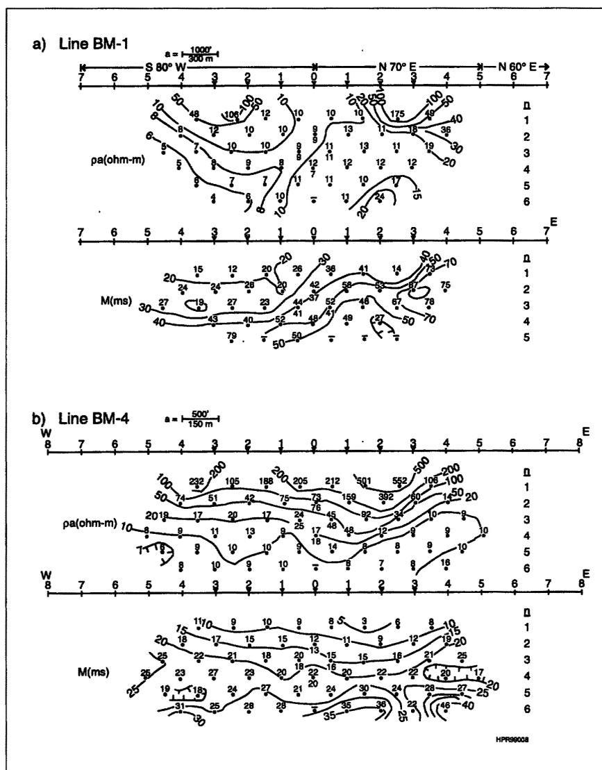
Figure 3. Observed apparent resistivity and induced polarization pseudosections: a) Line BM-1; and b) Line BM-4.
