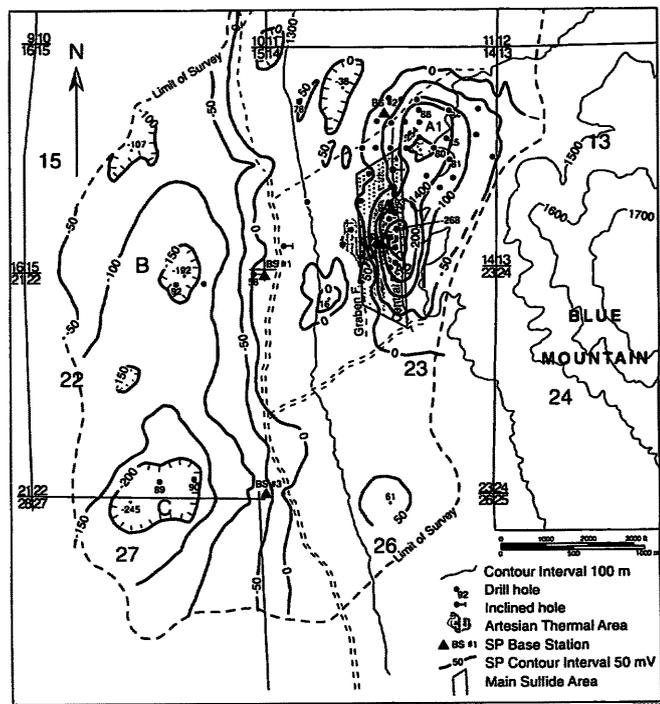
Figure 1. Self-potential survey, Blue Mountain geothermal area, Humboldt County, Nevada. The artesian thermal fluids and main mineralized body are likely sources for Anomalies A1, A2.
