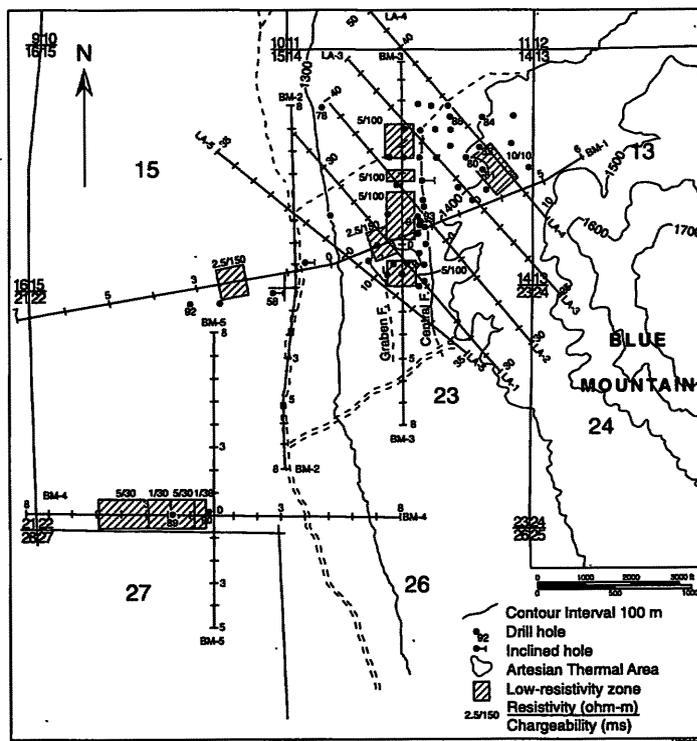
Figure 2. Resistivity/IP line locations, and low-resistivity areas determined by numerical modeling of Lines LA-4, BM-1, -3, -4. Compare with locations of the artesian thermal area and main sulfide body on Figure 1.
