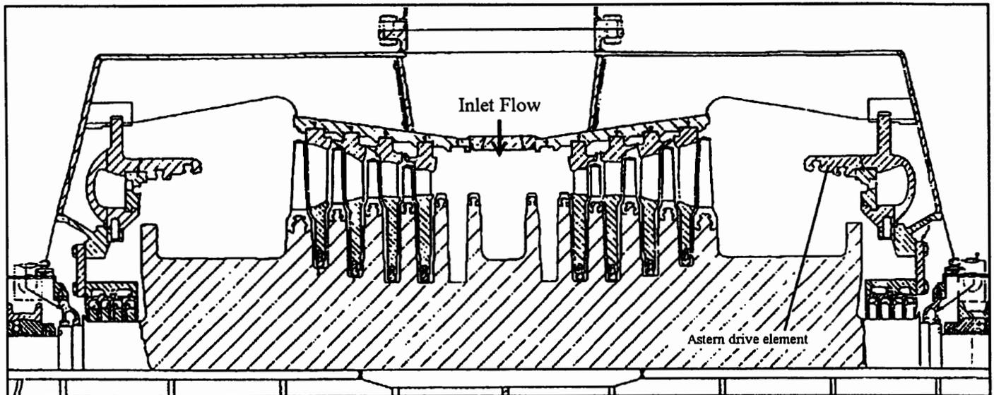
Figure 1. Geothermal turbine before uprate.
