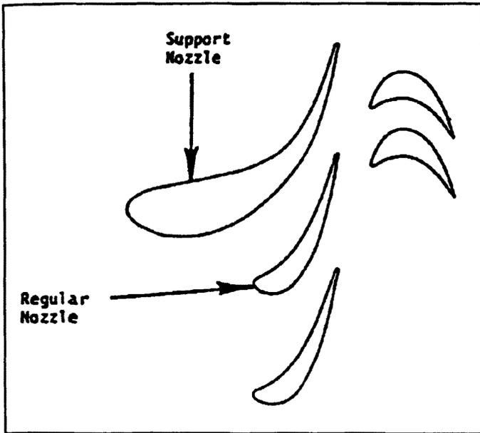
Figure 6. New high efficiency stage design.
