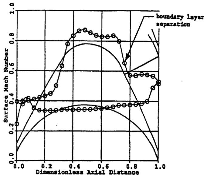
Figure 3. Mach number distribution. Typical of Early Bucket Design
