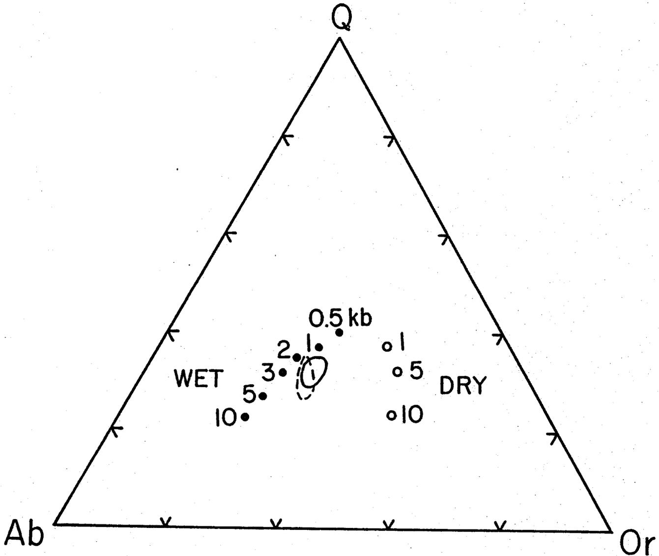
Figure A-12. Normative quartz - albite - orthoclase diagram showing compositions of Cuffytown Creek surface samples (solid line) and core samples (dashed line). Experimentally determined minima are from Tuttle and Bowen, 1958, Luth et al., 1964, and Luth, 1969.
