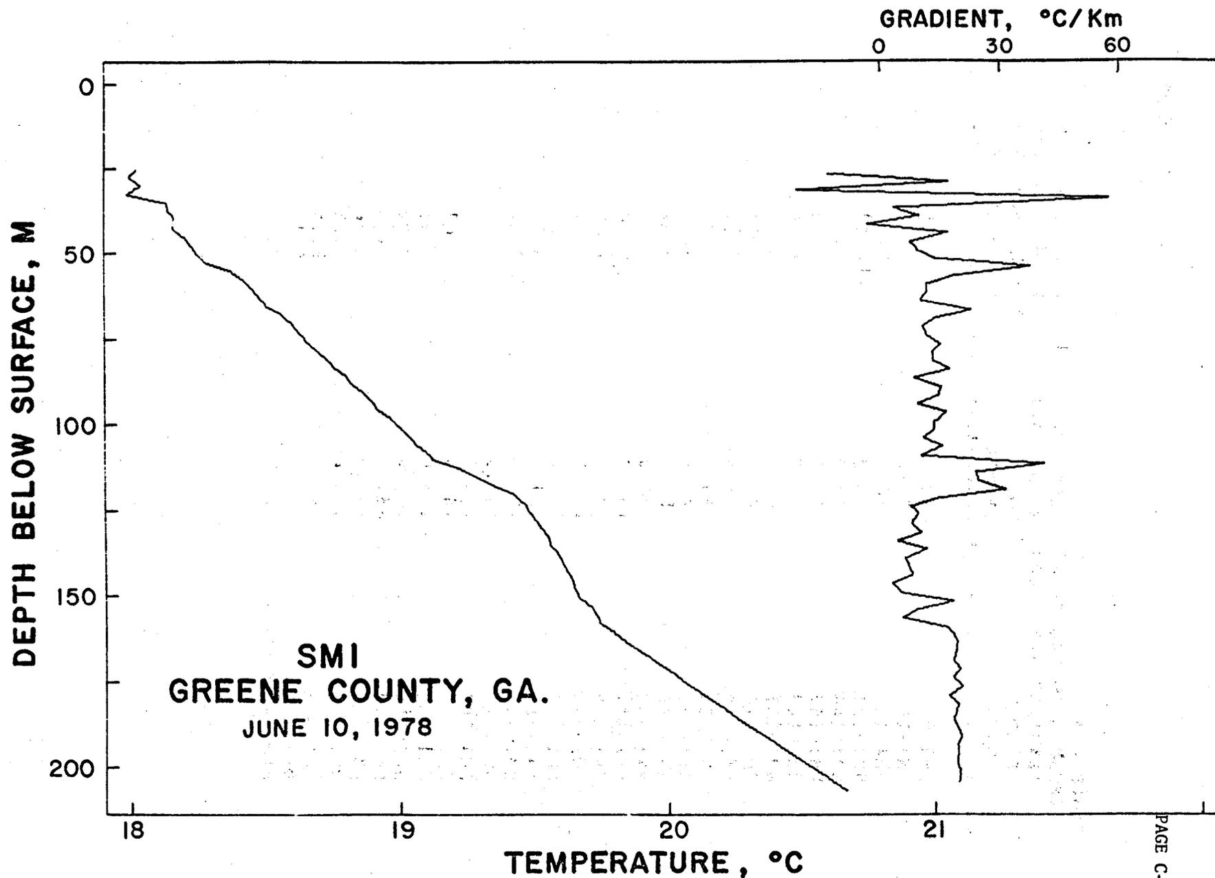
Figure C-3.2. New heat flow value of Hole SMI in the Siloam granite.
