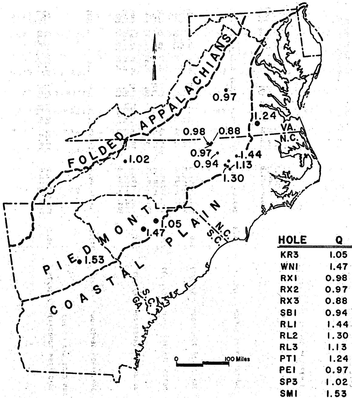
Figure C-3.1. Locations of holes drilled to date by VPI&SU and summarizes heat flow values.
