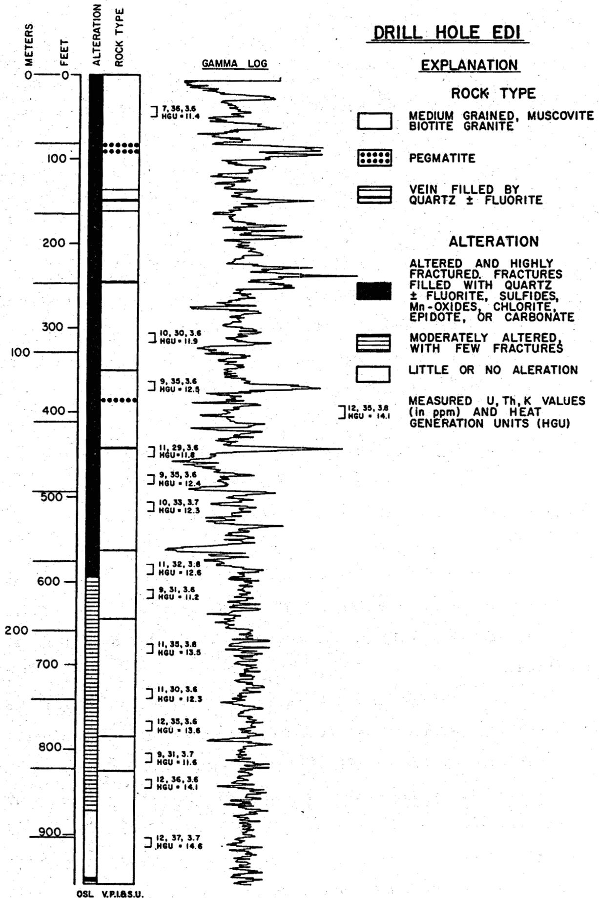
Figure A-11. Lithologic and gamma log of the EDI drill hole.
