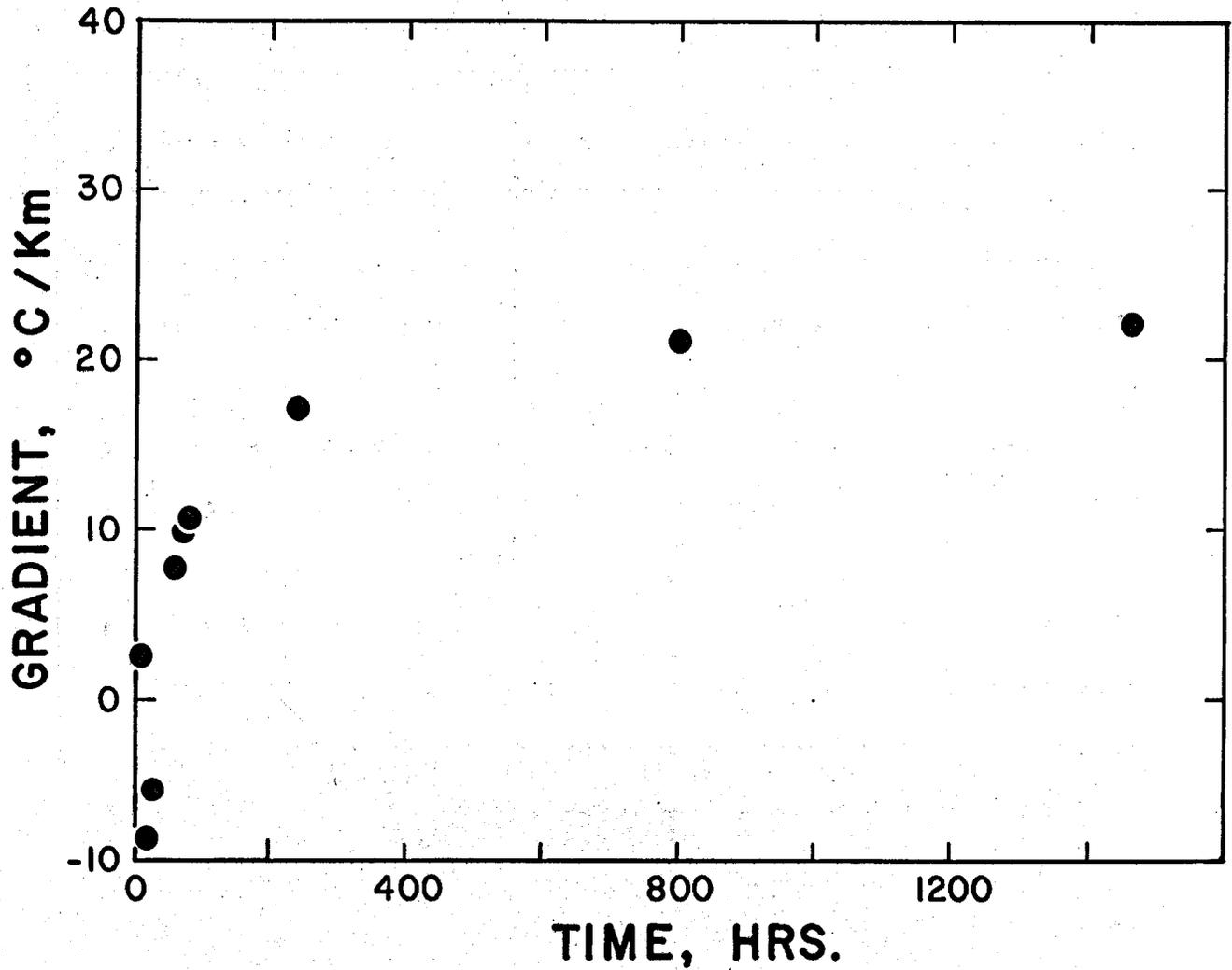
Figure C-2.1. Plot of gradients vs time since completion in hole C40, Fort Monmouth, NJ.
