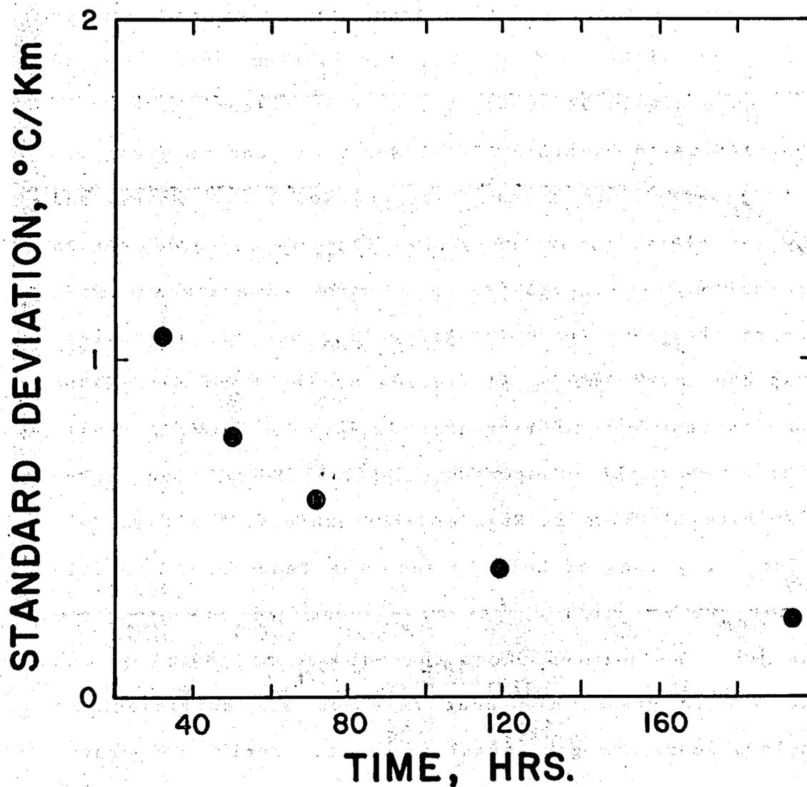
Figure C-2.3. Standard deviation of gradient versus time for hole C41, Sea Girt, NJ.
