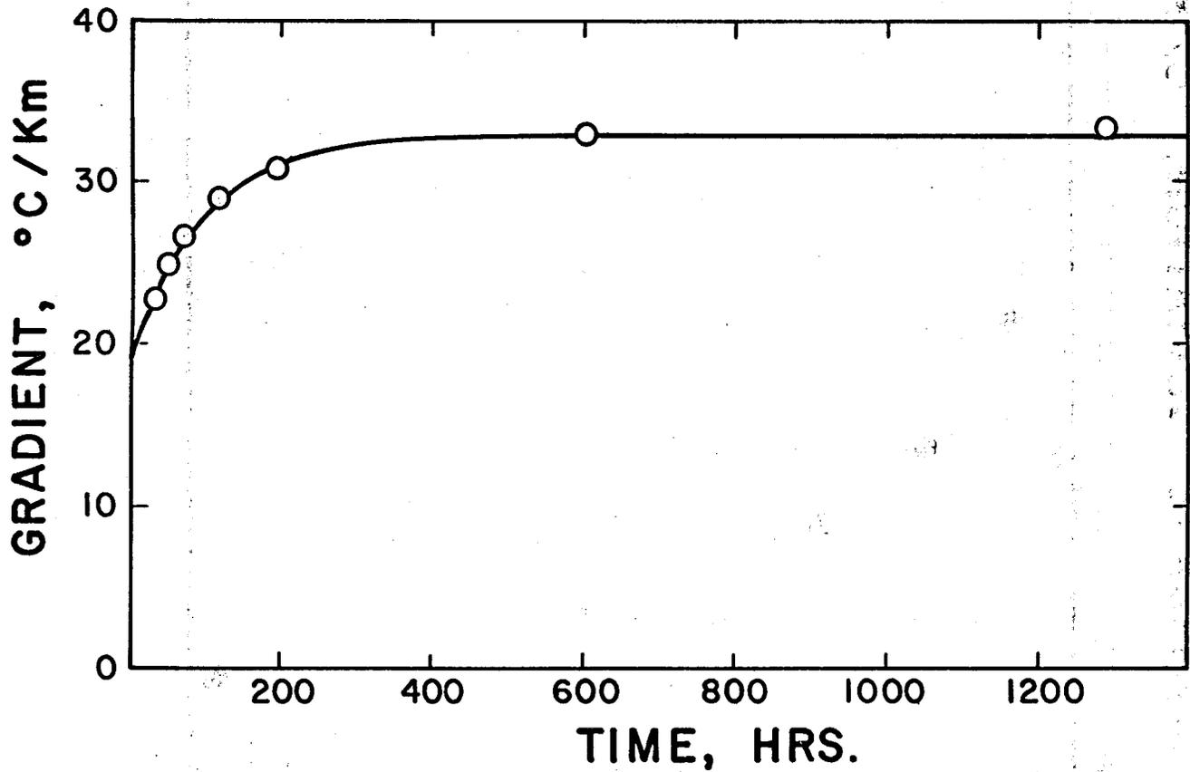
Figure C-2.2. Plot of gradient versus time since cementing in hole C41, Sea Girt, NJ. Solid line shows exponential cooling curve with the form of gradient =  $32.9^{\circ}\text{C}/\text{km} - 13.75 \text{ Exp}(0.010327 \text{ xt})$ .
