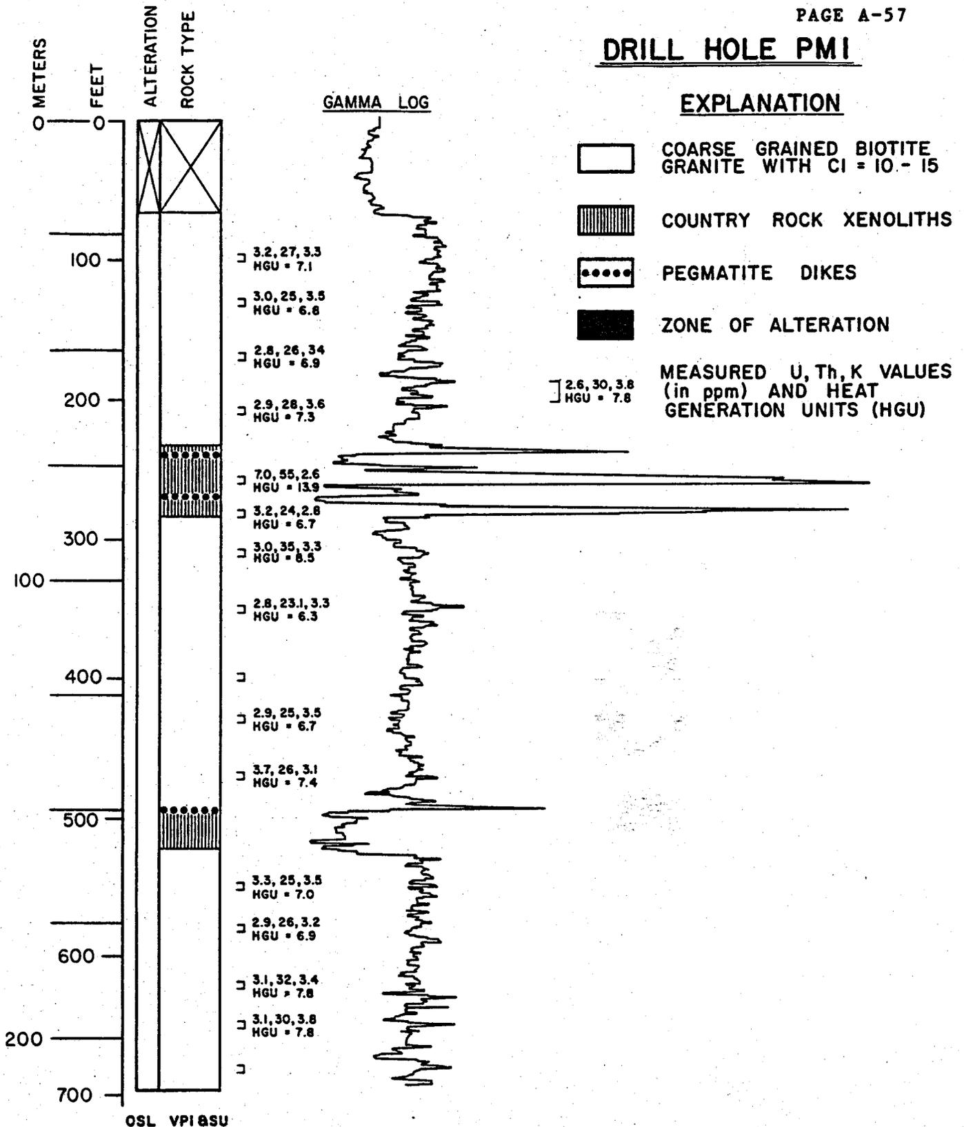
Figure A-5. Lithologic log of drill hole PMI, with corresponding alteration and gamma ray spectrometer log. Radioactivity measurements increase to the right.
