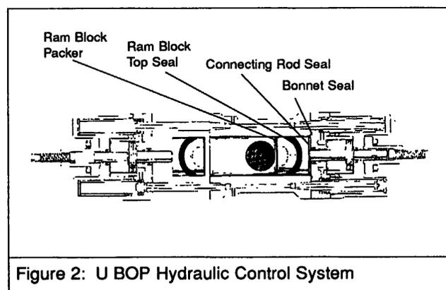
Figure 2: U BOP Hydraulic Control System
