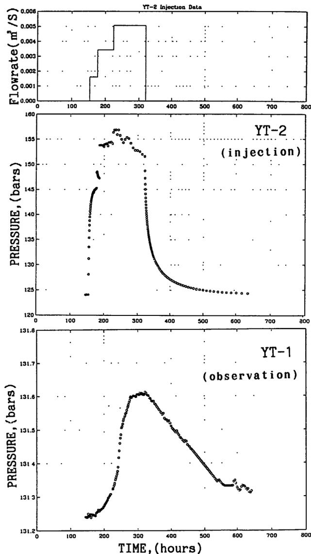
Figure 1. Injection rate (top panel) and pressure record (middle & bottom panels) for the multi-rate injection test of well YT-2 and YT-1 (YT-2; injection well, YT-1; observation well)
