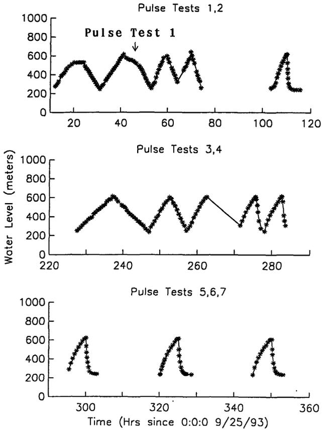
Figure 2. Water levels (depth of water table below the wellhead) recorded by an echometer in Well YT-2 during pulse tests
