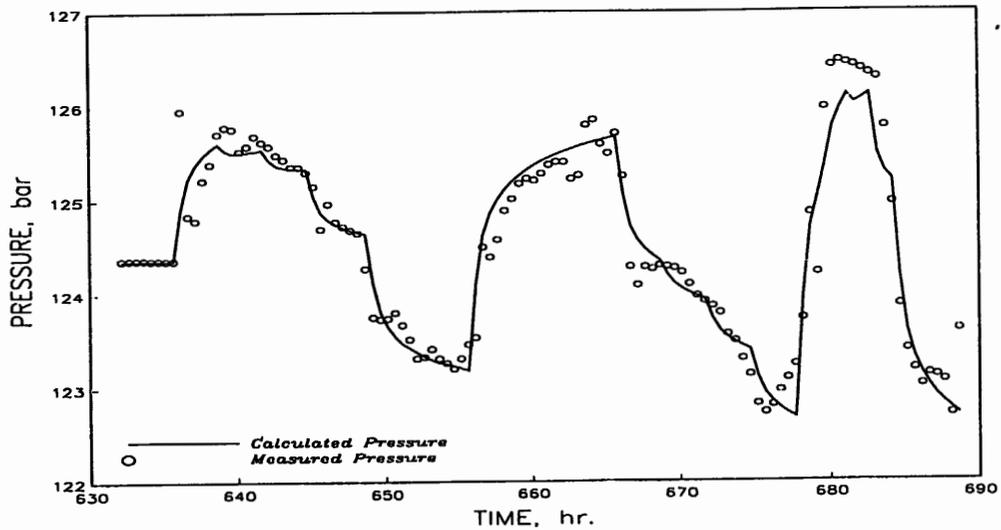
Figure 5. Comparison between measured (O) and computed (—) pressures for the first 3 cycles of pulse test 1 of YT-2
