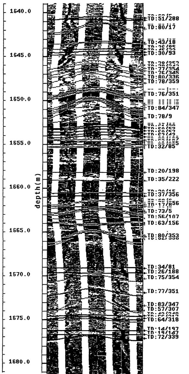
Figure 6. Schlumberger's FMI log image from 1640m to a depth of 1680m of well YT-2. sine wave; fracture, TD; true dip (magnitude/azimuth)
