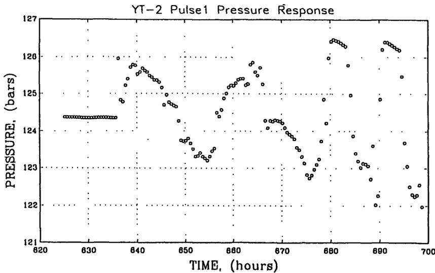
Figure 3. Pressure record of well YT-2 during "pulse test 1"
