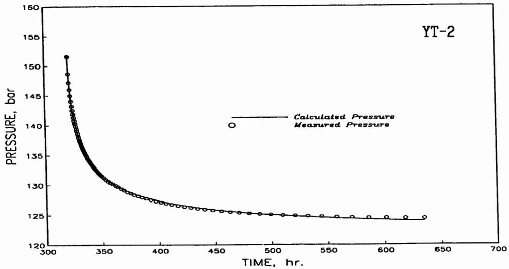
Figure 4b. Comparison of measured (O) and computed (—) fall-off pressures in well YT-2 for the multi-rate injection test.
