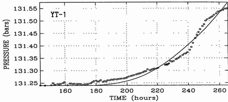
Figure 4a. Comparison of measured (O) and computed (—) pressure response of well YT-1 to injection into YT-2
