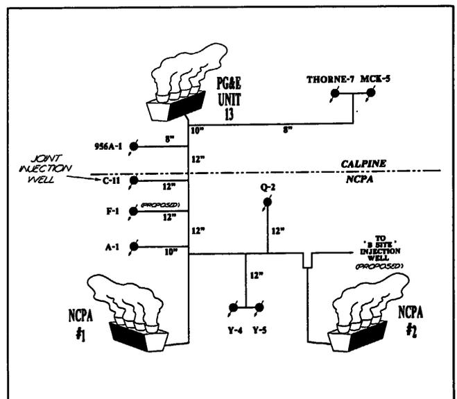
Figure 3. Injection schematic.
