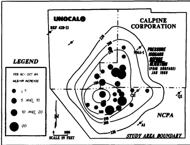
Figure 8. Location of wells with flow rate increases due to injection.
