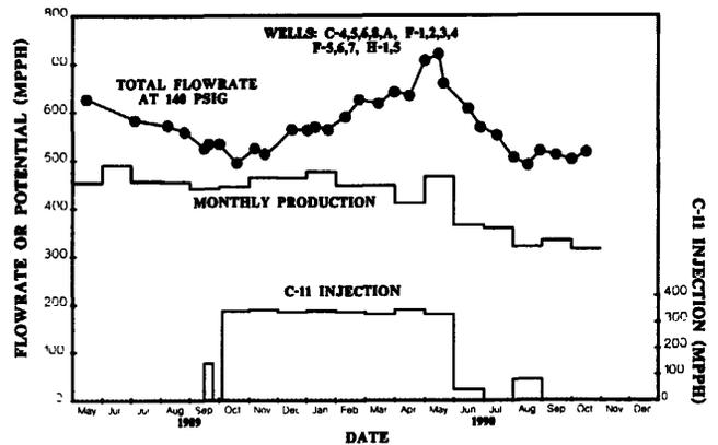
Figure 10. Total flow rate of NCPA wells, offset to injector C-11.
