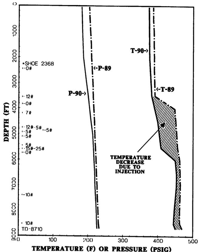
Figure 16. C-11 temperature and pressure survey on September 20, 1989 - 1/2-inch vent; survey on August 17, 1990 - 3-inch vent.
