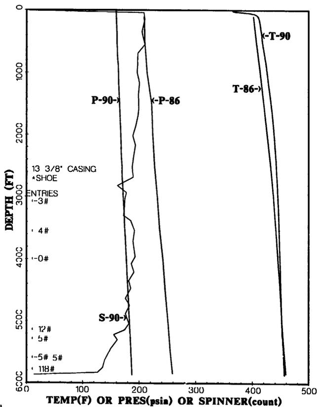
Figure 15. Pressure and temperature comparison, Well F-6, 1986 and 1990.
