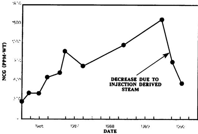
Figure 14. Well F-5, noncondensable gases vs. time.
