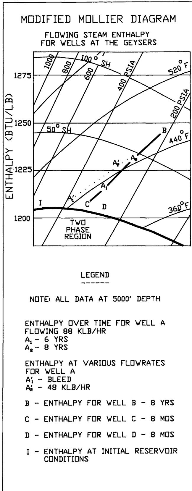
Figure 3. Increasing enthalpy trend (at 5,000 ft. depth) is linear for a "typical" southeast well as reservoir becomes more depleted. Well D shows initial conditions of a "wet" well. Well A exhibits an essentially isothermal pressure increase as its flowrate was reduced (Line A<sub>2</sub>-A<sub>1</sub>).
