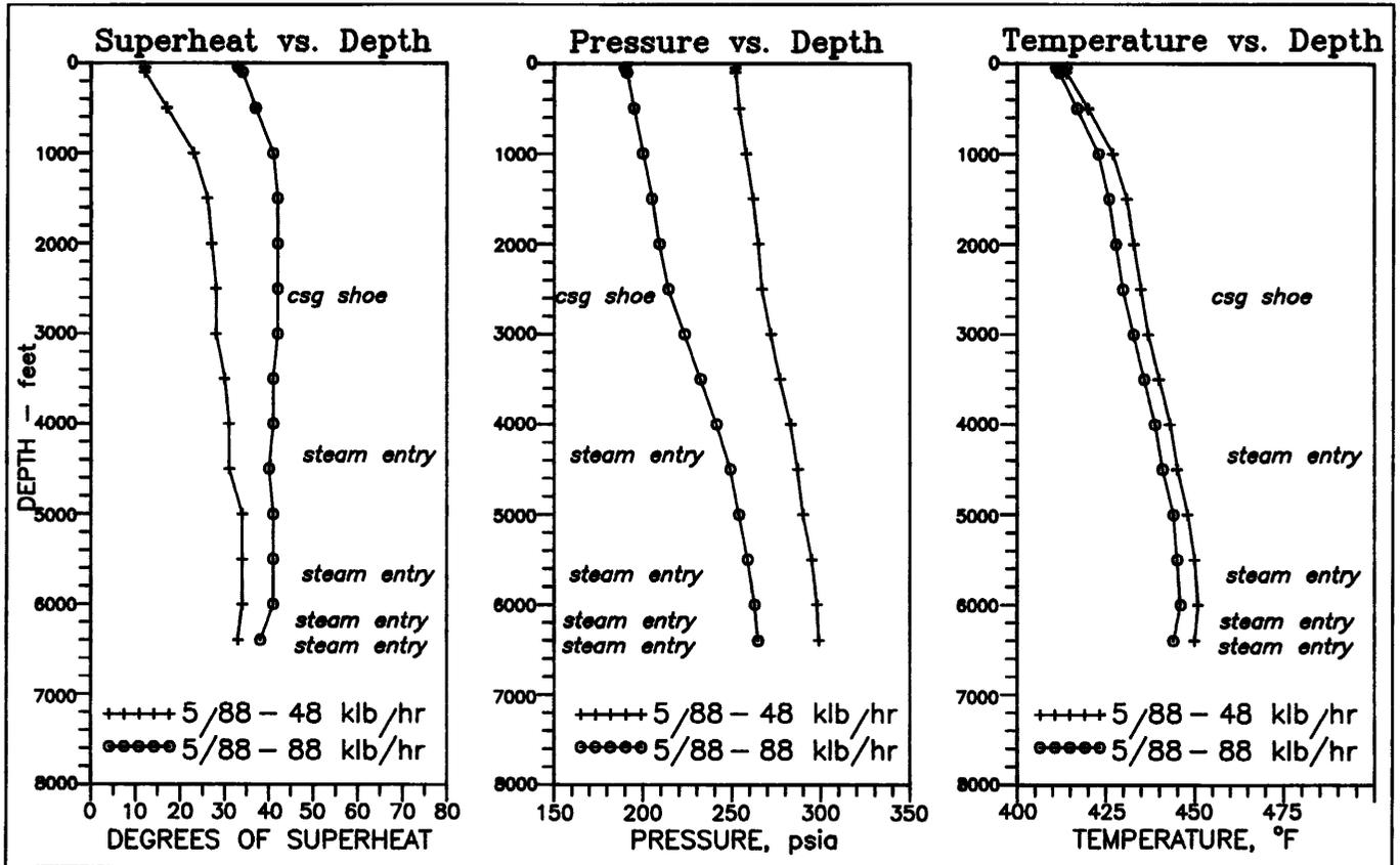
Figure 4. Comparison of superheat, pressure and temperature vs. depth for well A at full flow (88 klb/hr) and half flow (48 k lb/hr). Well A exhibits an increase in superheat gradient controlled by a decrease in the pressure gradient at the lower flow rate.
