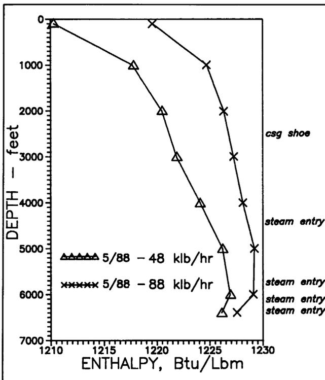
Figure 5. Comparison of enthalpy vs. depth for well A at full flow (88 klb/hr) and half flow (48 klb/hr). Well A exhibited an increase in enthalpy gradient and higher heat loss in the cased portion of the wellbore as its flowrate was reduced.
