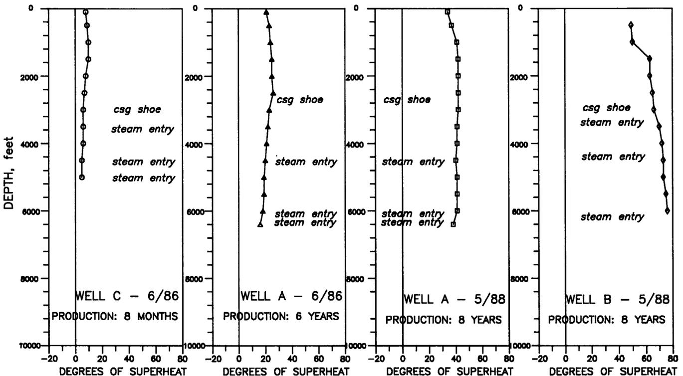
Figure 2. Evolution of superheat vs. depth over time. Increasing superheat trend is observed as reservoir becomes more depleted.
