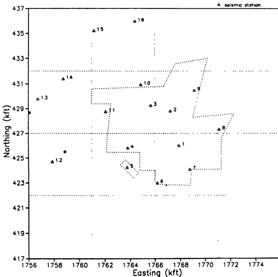
Figure 10. The digital array of 16, 3-component bore hole stations being used to monitor the seismicity of the northwest Geysers region by the Coldwater Creek Operating Company (Weiser, 1989).
