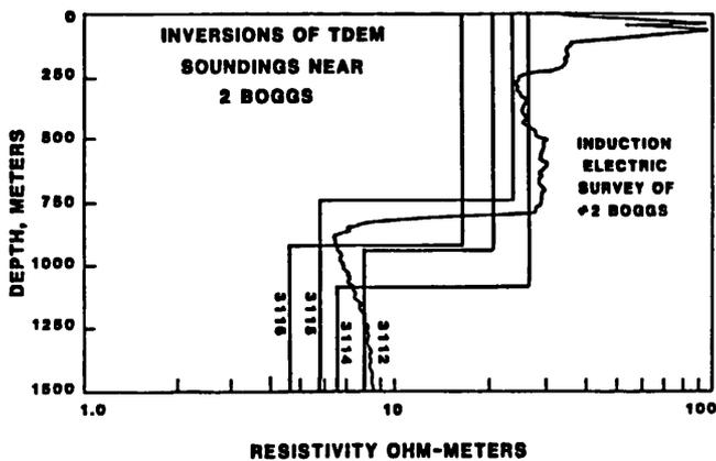
**Figure 7.** Inversions of four TDEM soundings from Boggs Mountain (Figure 4) and induction electric log from Boggs No. 2 well. Reproduced from Keller and others (1984).
