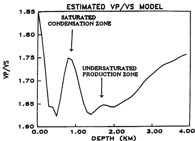
Figure 12. A VP/VS model obtained by O'Connell (1986) using MEQs in the main production zone at The Geysers.
