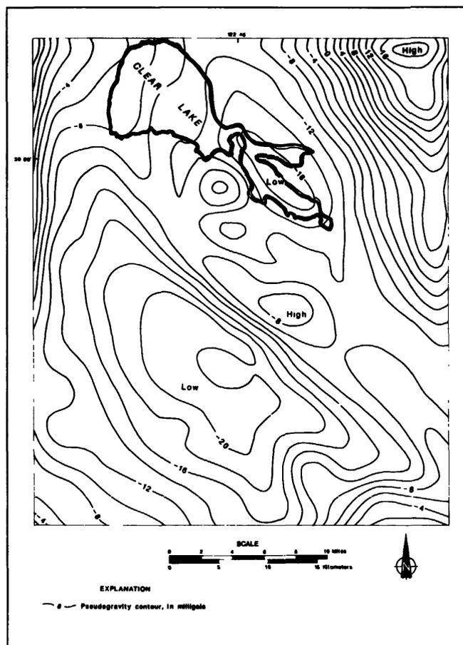
**Figure 3.** The Geysers area showing pseudogravity derived from filtered aeromagnetic data (5-km cutoff); density contrast, 0.15 g/cm<sup>3</sup>; magnetization contrast, 0.003 cgs units; Contour interval, 2 mGal. (From Isherwood (1975).
