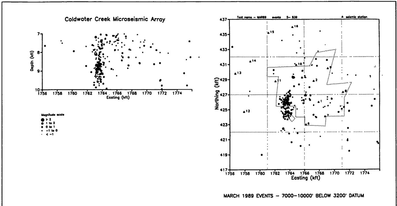
Figure 11. Cross section (left) and plan view (right) of events ( $M \geq -1$ ) located by array in Figure 10, for a one-month period of 1989 during an injection period (Weiser, 1989).
