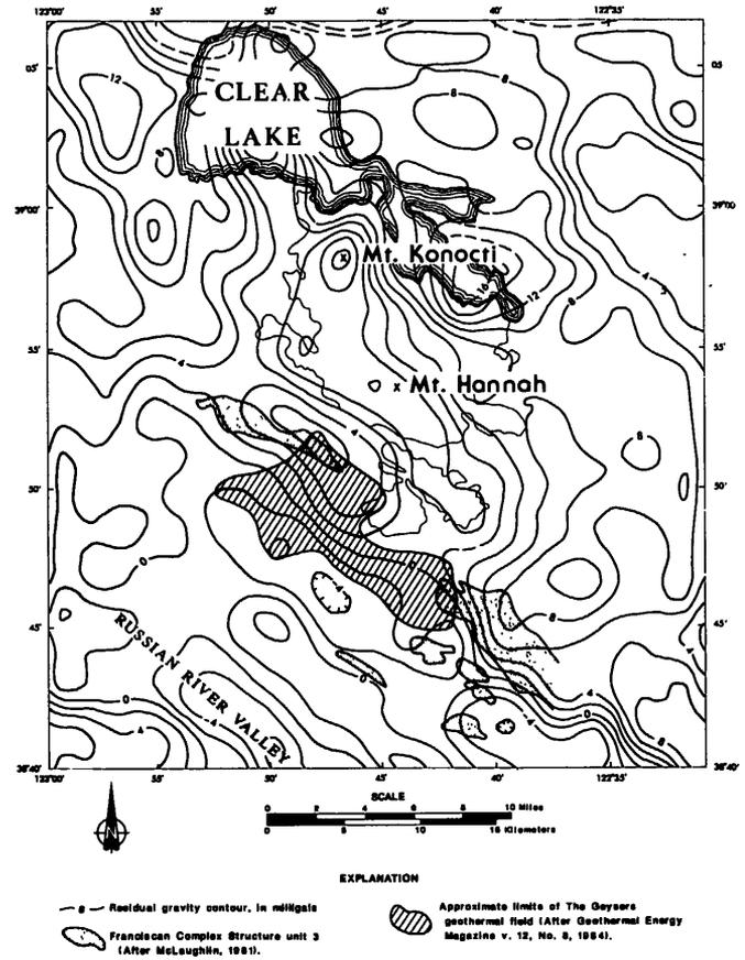
Figure 2. Residual gravity (at  $2.67 \text{ g/cm}^3$ ) in the vicinity of The Geysers geothermal field, after removal of the field from a sphere buried at 13.5 km. Contour interval 2 mgal. After Isherwood (Figure 16, 1975).
