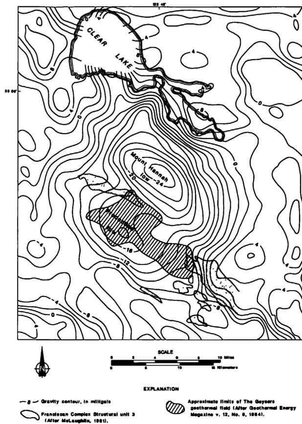
Figure 1. The Geysers area, California, showing residual gravity based on reduction densities of  $2.67 \text{ g/cm}^3$ . Contour interval, 2 mGal. From Isherwood (1975).
