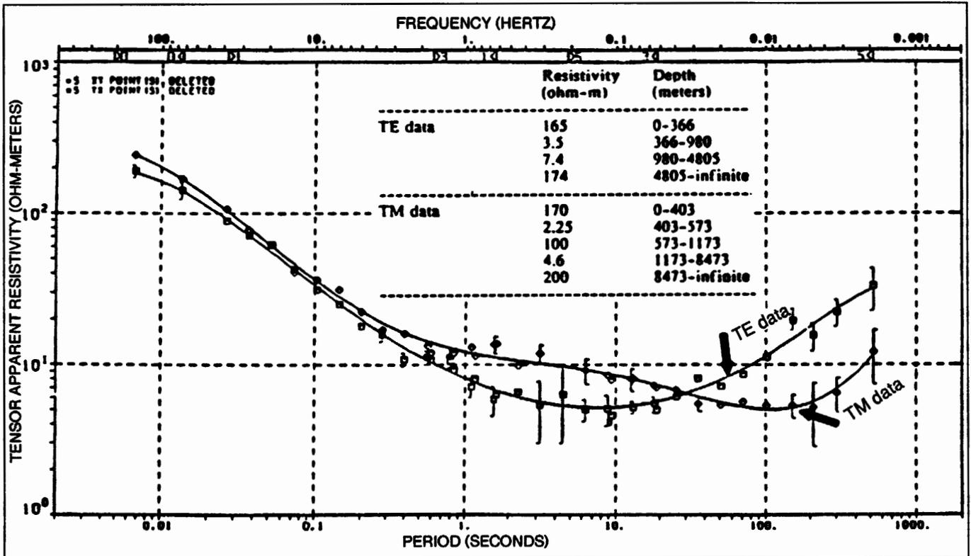
Figure 8. Sample MT sounding from Clear Lake volcanic field in Mount Hannah region (exact location proprietary). The error bars represent two standard deviations. TM and TE designations for data curves are discussed in text. Layered models for the TE and TM data are shown in the inset table.
