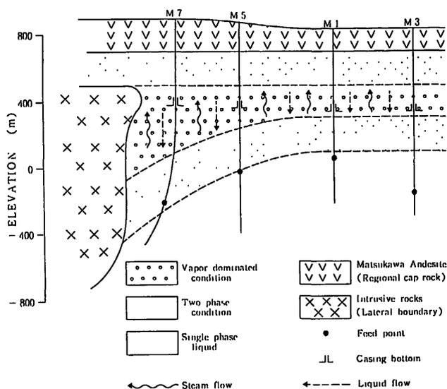
Fig. 4 Conceptual model of the initial state of the Matsukawa geothermal reservoir (after Hanano and Matsuo, 1990).
