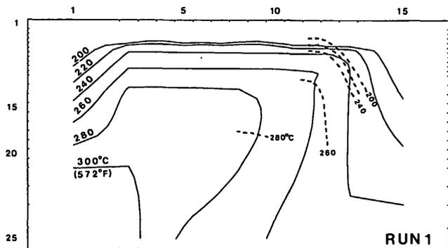
Fig. 6 Temperature distribution at 50,000 years of the final model, along with initial temperature distribution (dashed line) (after Hanano, 1992).
