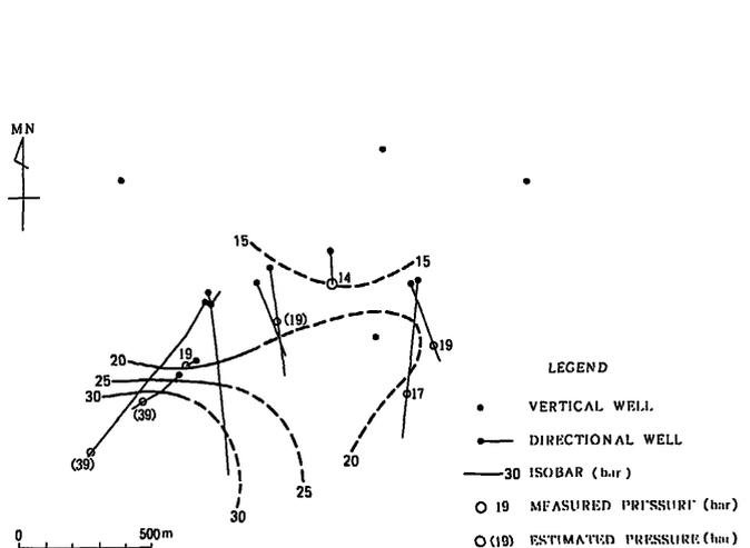
Fig. 3 Shut-in pressure distribution at feed points in October 1988 (after Hanano et al., 1989). Pressures are absolute.
