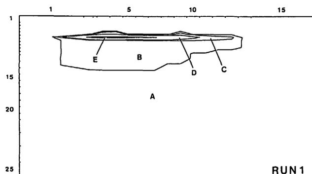
Fig. 7 Distribution of water saturation at 50,000 years of the best model (A :  $S_w=1.0$  ( $k_{rs}=0.0$ ), B :  $0.95 < S_w < 1.0$  ( $k_{rs}=0.0$ ), C :  $0.84 < S_w < 0.95$  ( $k_{rv} > k_{rs} > 0.0$ ), D :  $0.5 < S_w < 0.84$  ( $0.99 > k_{rs} > k_{rv}$ ), E :  $S_w < 0.5$  ( $k_{rs} > 0.99$ )) (after Hanano, 1992).
