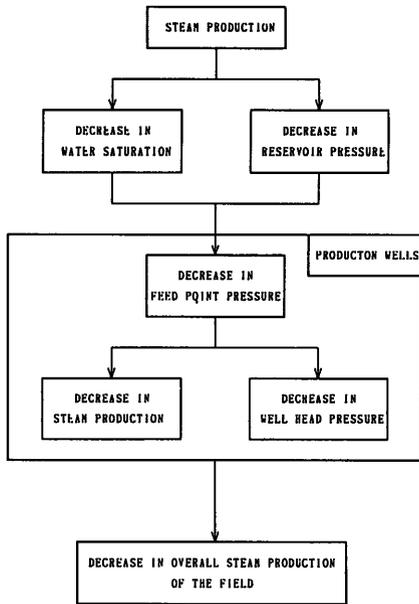
Fig. 8 Mechanism of decline of steam production in vapor-dominated geothermal fields.
