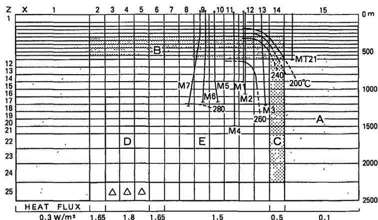
Fig. 5 Grid mesh with initial temperature distribution, along with permeability distribution (A =  $5 \times 10^{-17} \text{ m}^2$ , B =  $1 \times 10^{-13} \text{ m}^2$ , C =  $5 \times 10^{-14} \text{ m}^2$ , D =  $1 \times 10^{-13} \text{ m}^2$ , E =  $1 \times 10^{-15} \text{ m}^2$ ), location of mass input ( $\Delta$ ), and conductive heat input of the final model of natural state simulation of the Matsukawa geothermal reservoir (after Hanano, 1992).
