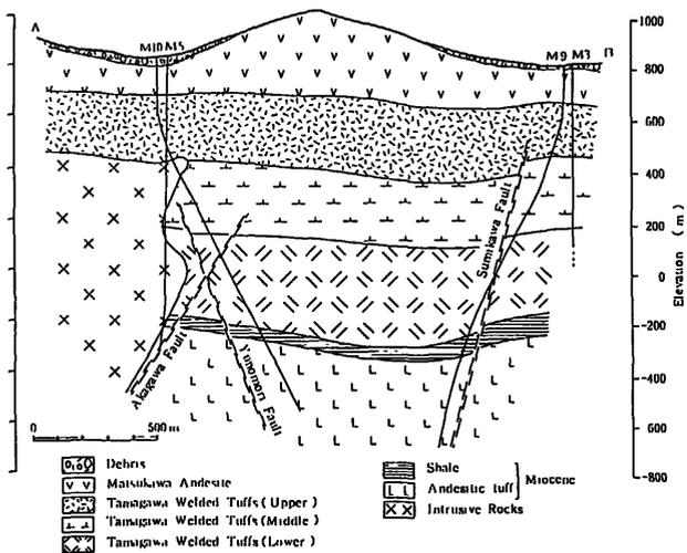
Fig. 2 Geological cross section of Matsukawa (after Akazawa and Muramatsu, 1988). Location of the cross section is shown in Fig. 1.
