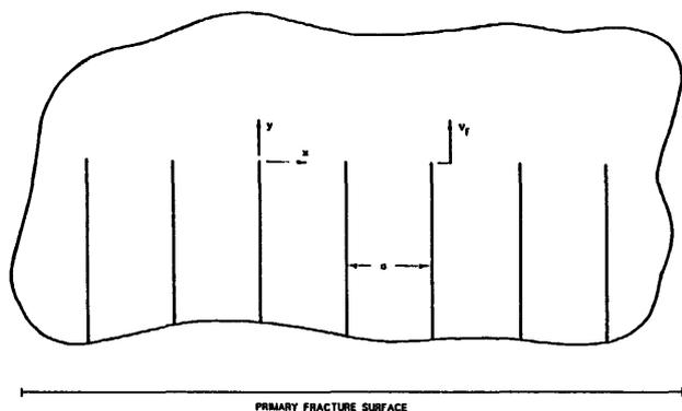
3b. Simplified model of secondary fractures as infinite array of parallel, semi-infinite cracks with spacing  $s$  and propagation  $V_F$  (Barr & Cleary, 1980). This assumption of a stable array was verified by stability analysis.
