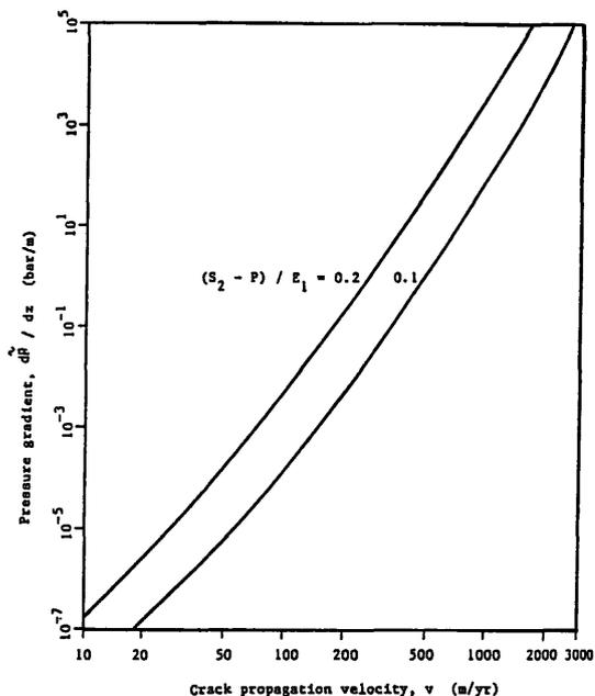
3c. Sample calculations of secondary crack growth speeds  $V_F$  illustrating the dominant dependence on the pressure-gradient driving convective fluid flow (Barr & Cleary, 1980).
