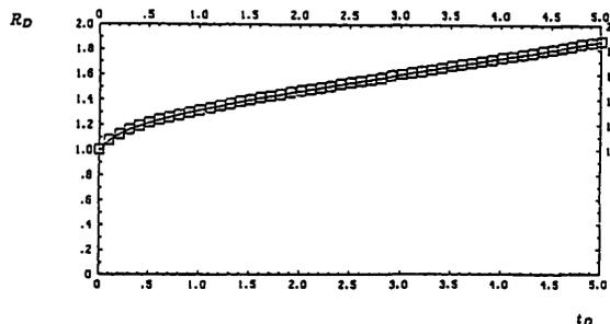
4b. Illustration of calculations for dimensionless crack growth vs. dimensionless time,  $R_D$  vs.  $t_D$  under PPIC conditions. The associated excess pressure is  $(p_F - \sigma_c) / \sigma_c = \sigma_D$ . [Dimensionless quantities are defined by Vogeler et al., 1985.]
