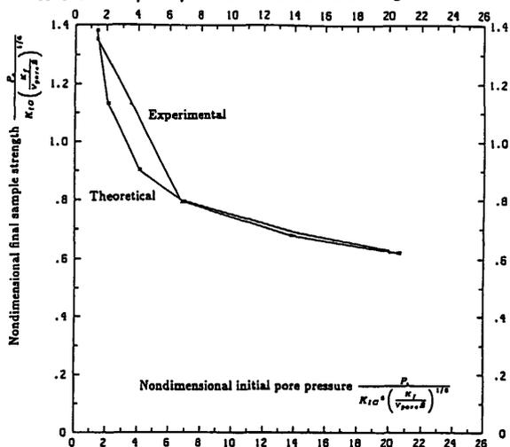
4c. Comparison of model predictions vs. measured strength of samples in Brazilian tests after being subjected to PPIC process in Figure 4a (taken from Vogeler et al., 1985).
