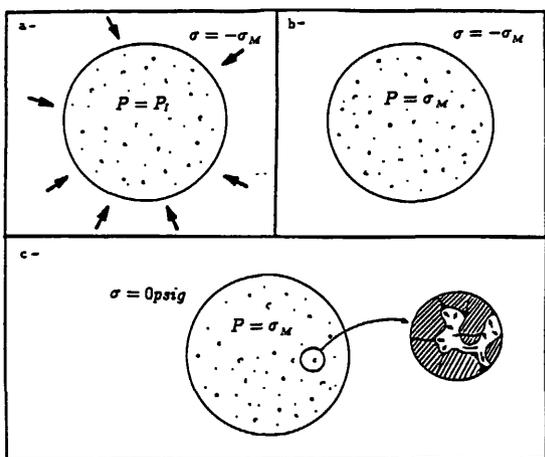
a- Before permeation  $\sigma_{eff} = P_i - \sigma_c$       b- At saturation  $\sigma_{eff} = 0$
