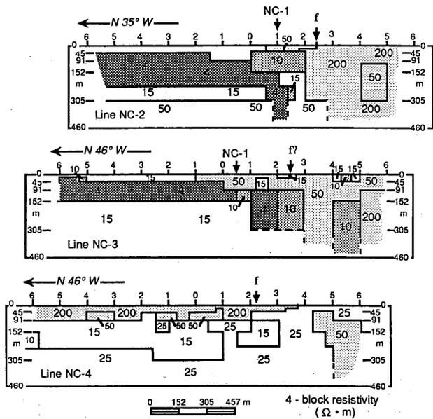
Figure 5. Numerical model solutions for Lines NC-2, NC-3, and NC-4. The low resistivity bodies (shaded) are interpreted as the fluid conduits and outflow plume.
