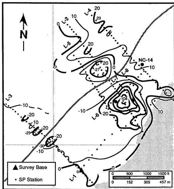
Figure 7. Self-potential map for the Newcastle geothermal area. All values are referenced to the base station at the intersection of Lines 1 and 3.
