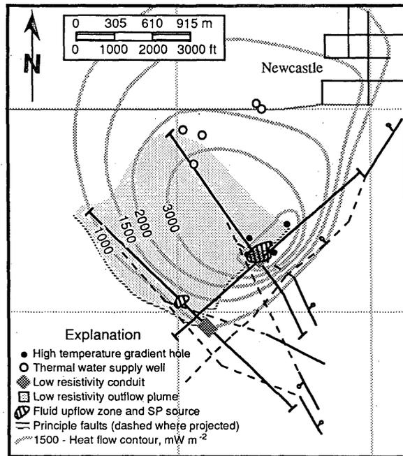
Figure 9. Interpretation summary showing probable fluid conduits indicated by resistivity and SP data, the outflow plume, and faults projected beneath alluvium.
