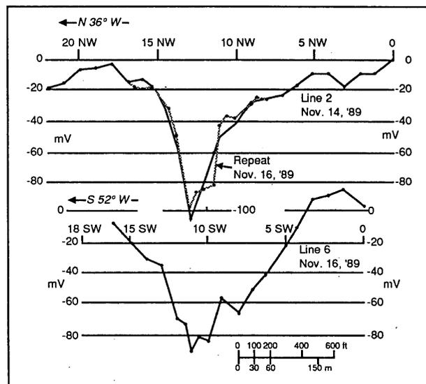
Figure 8. Self-potential profiles for Lines 2 (northwest) and 6 (northeast) across the SP minimum. Data for a repeat profile on Line 2, recorded two days later, are also shown.
