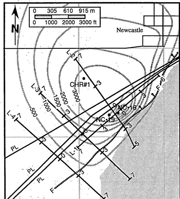
Figure 2. Location of resistivity profiles with respect to heat flow anomaly, high temperature gradient holes, Antelope Range fault, and high voltage transmission lines. Outcropping volcanic rock is shown as a shaded pattern.
