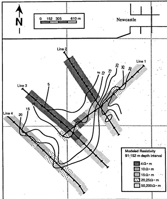
Figure 6. Contoured third separation ( $n = 3$ ) apparent resistivity and modeled intrinsic resistivity for the depth interval 91-152 m.
