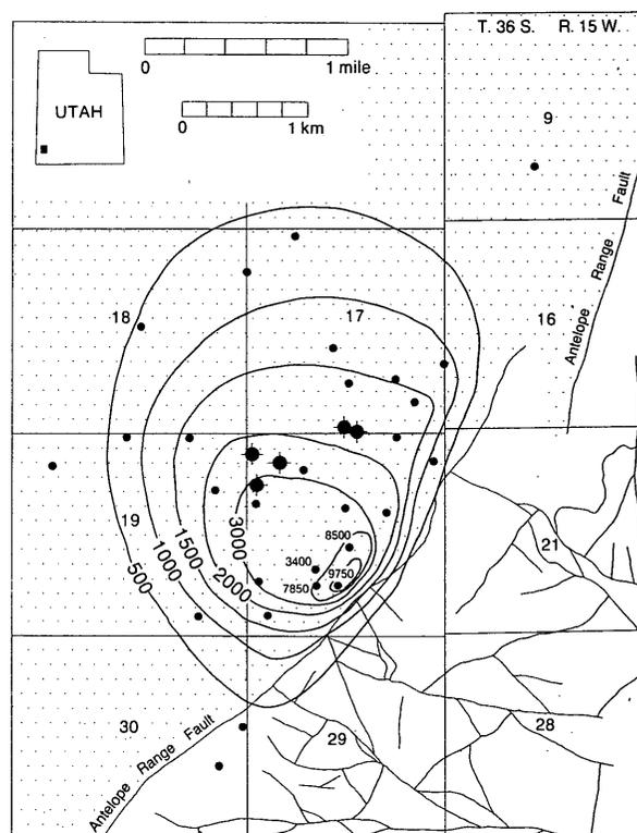
Figure 1. Location and heat flow distribution of the Newcastle geothermal area. Heat flow contours in  $mW m^{-2}$ . Large circles are thermal water supply wells, small circles are temperature gradient holes. Faulting within the range is indicated.
