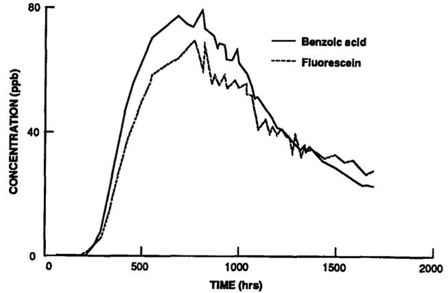
Figure 4. Measured concentrations of fluorescein and benzoic acid in the production fluid from well 76-7. The tracers were injected at time = 0 hours.
