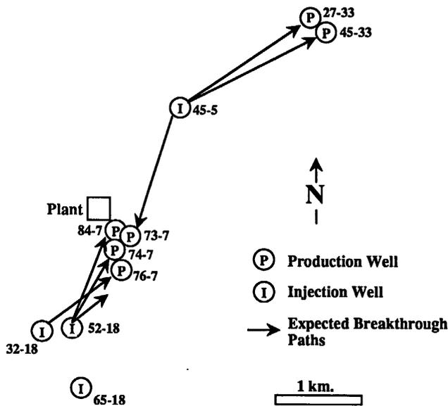
Figure 2. Bottom-hole well locations and expected breakthrough paths for the injected tracers.
