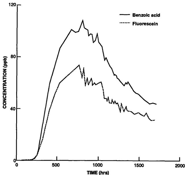
Figure 5. Hypothetical return curve in which tracers are corrected for thermal decay at the average temperature indicated by the tracer ratios.
