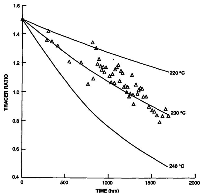
Figure 6. Actual tracer ratios in fluid from well 76-7 compared to ratios calculated with the assumption of constant temperature along the injection-production flowpath.
