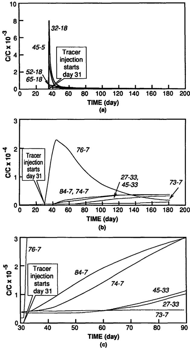
Figure 3. Predicted tracer concentrations in the injection wells (a) and the production wells (b), and predicted early time behavior in the production wells (c).
