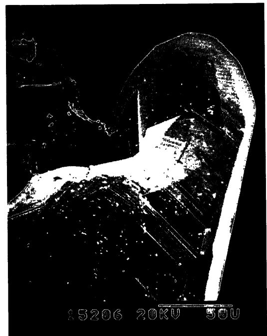
FIGURE 6. SEM PHOTOMICROGRAPH OF PYRRARGYRITE FROM A VEIN CUTTING QUARTZ-SERICITIZED RHYOLITE ASH-FLOW TUFF, COREHOLE VC-2B, DEPTH 351 M.
