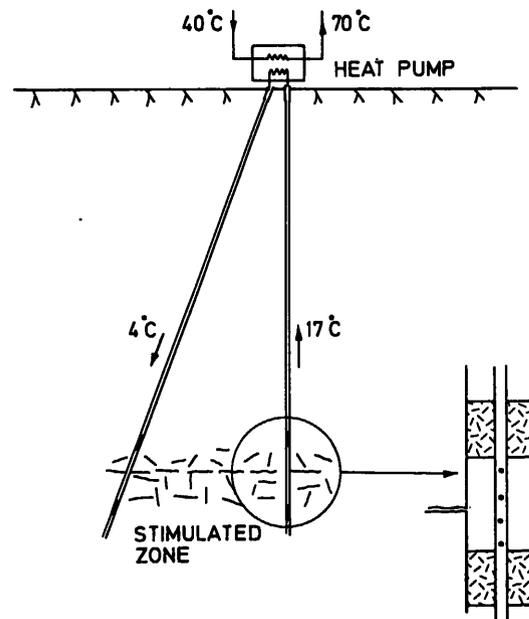
Figure 5. Principle of the Swedish HDR concept.
