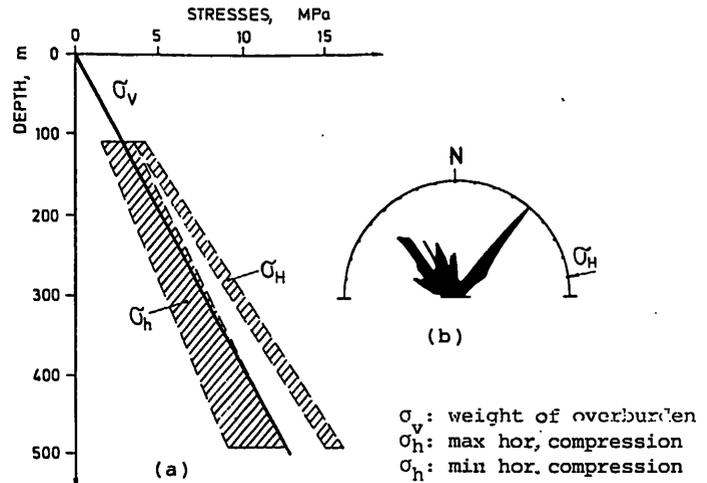
Figure 4 a) Magnitudes of the principal stresses as a function of depth.
