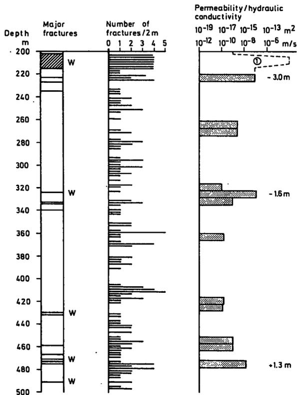
Figure 3 Plot showing major fractures, open fractures, fracture frequency, hydraulic conductivity and pressure heads in Fjb 1. W = naturally water conducting fractures (D) Evaluated from pump tests.
