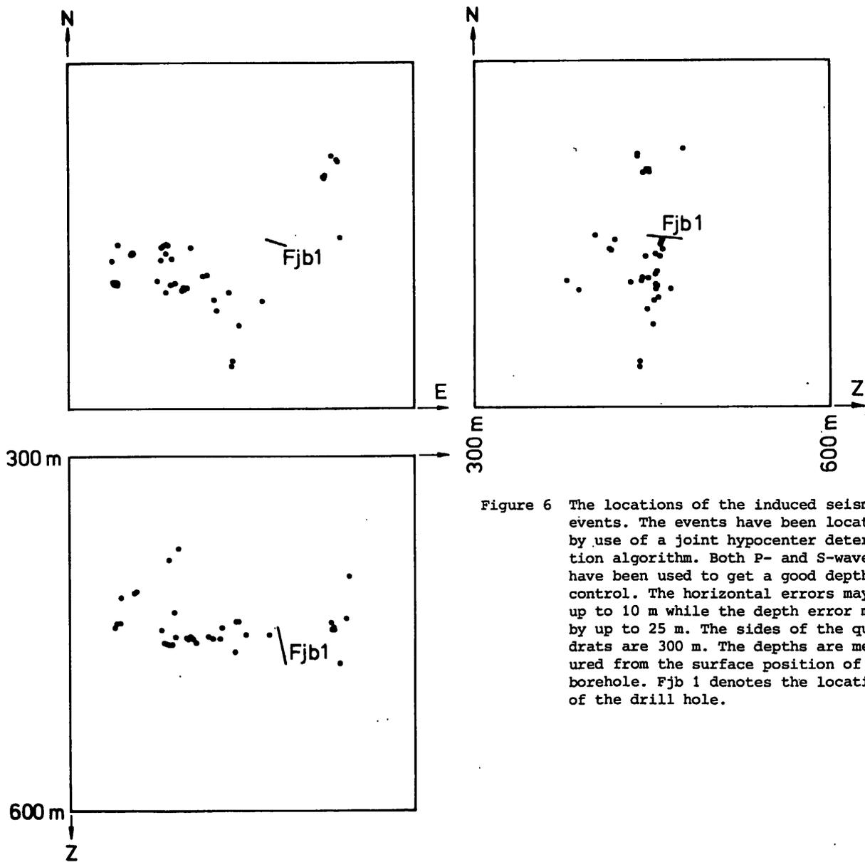
Figure 6 The locations of the induced seismic events. The events have been located by use of a joint hypocenter determination algorithm. Both P- and S-waves have been used to get a good depth control. The horizontal errors may be up to 10 m while the depth error may be up to 25 m. The sides of the quadrats are 300 m. The depths are measured from the surface position of the borehole. Fjb 1 denotes the location of the drill hole.
