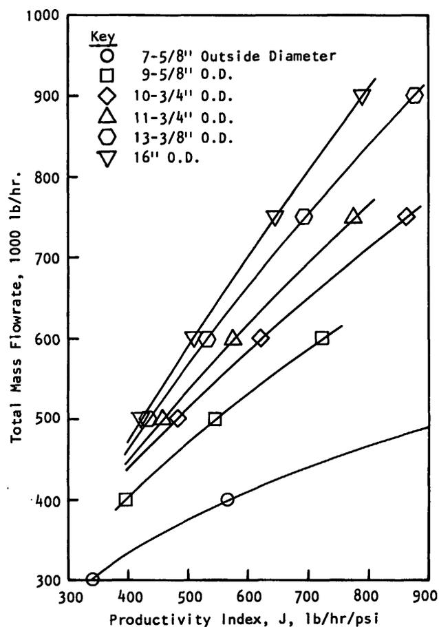
Figure 1. Computer Model Results of Flowrate vs. Productivity Index.
