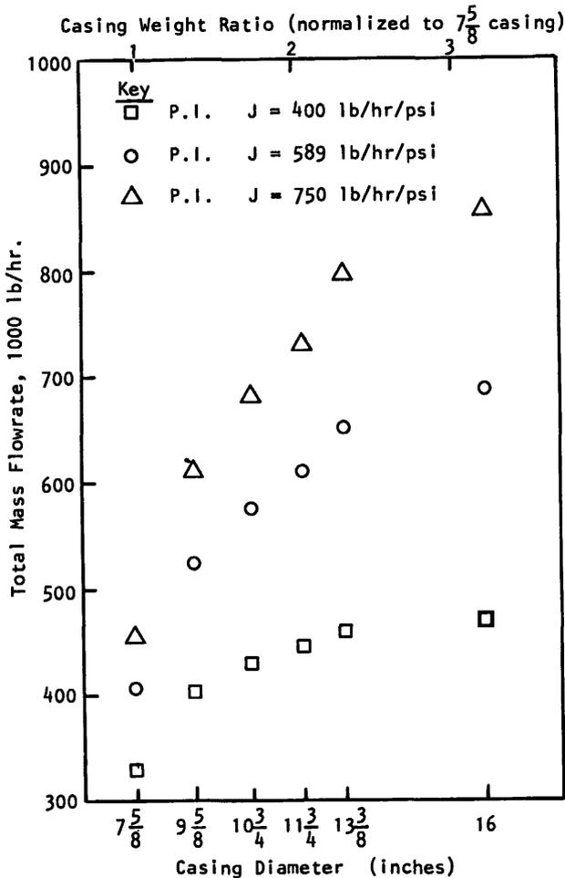
Figure 2. Flowrate as a Function of Casing Diameter & Productivity Index.
