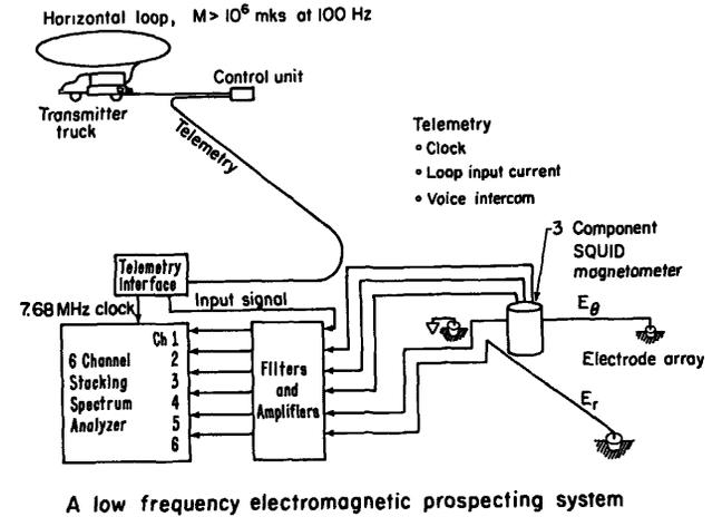
A low frequency electromagnetic prospecting system
