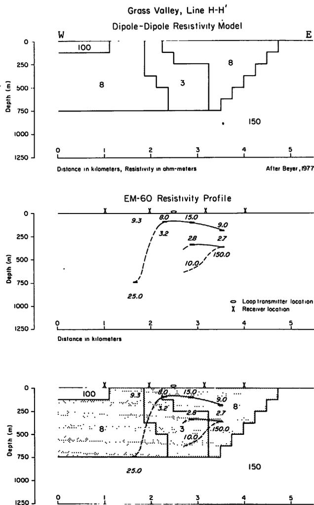
Figure 7. Resistivity cross section over line H-H' in Panther Canyon (a) two-dimensional dipole-dipole resistivity model (b) profile of one-dimensional EM-60 electromagnetic soundings; (c) comparison of parts a and b.
