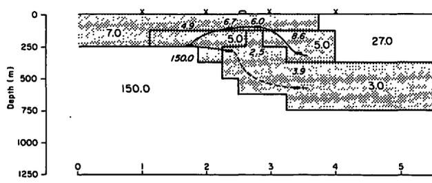
Figure 6. Resistivity cross section over line H-H' in Panther Canyon (a) two-dimensional dipole-dipole resistivity model (b) profile of one-dimensional EM-60 electromagnetic soundings; (c) comparison of parts a and b. XBL 802-6775
