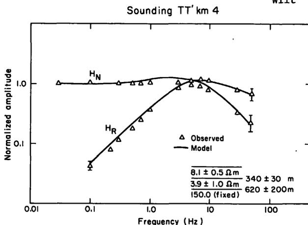
Figure 5. Normalized magnetic field amplitude spectra normal and radial fields sounding TTS Panther Canyon. XBL 802-6816
